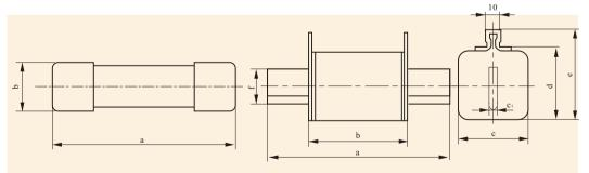
Chart 10 RT14 dimension 22\*58 Dimensions of tubular cylinder hat-shape type of fuse combination Chart 11: NT00, NT1, NT3 The dimensions of the knife-shaped fuse combination units
