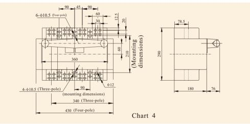
■ SG1-1000A~1600A outer-box operation panel drill dimensions
