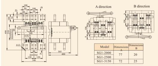
Notes: SG1-2000A~3150A without rear-board wiring, four-pole not available temporary
