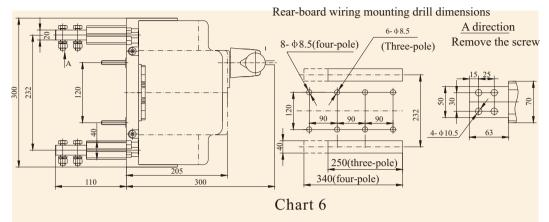
$\odot$  SG1-1000A  $\sim$  SG1-1600A rear-board wiring overall and mounting dimensions
